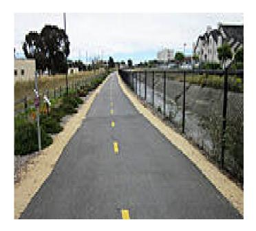
The Centennial Way Trail follows the path of the BART line between San Bruno station and South San Francisco station. The BART, of course, runs underground while the trail doesn't. The 10-foot-wide trail is paved with asphalt and has 2-foot granite shoulders. It meanders through a low-maintenance landscaped area, with wildflowers, and is lit for night use. Street crossings are made easy with pedestrian signals at Spruce and Chestnut avenues and inground flashing lights at Orange Avenue.
